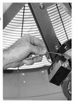
raise it up, then slip the belt from the motor pulley.
