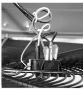
The red wire should plug into position 3 on the switch (closest to the grille center), while the remaining black wire should plug into position 1 (farthest from the grille center) on the switch.
