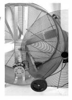
Loosen the bolts holding the motor to the struts using a 9 mm or crescent wrench. Do not remove the bolts completely. Once bolts are loose, place your hand underneath the motor and
