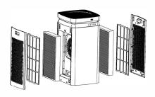
4. Remove all packing materials on the filter screen and put the filter screen back into the purifier.
