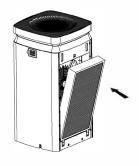
5. Re install the side cover, align and insert the fixed groove, and then push the side cover close to the machine, and the side cover will pull in automatically.
