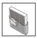
2. Install the composite filter into the machine.
