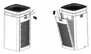
When re installing the side panel cover, align and insert the fixed groove, push the side panel cover close to the machine, and the side panel cover will automatically close to the machine.
