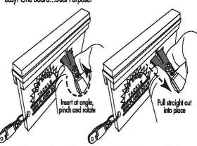
Assembly shown above is for running your board off your port side. Simply reverse the direction of the bracket to run the board off the starboard side
