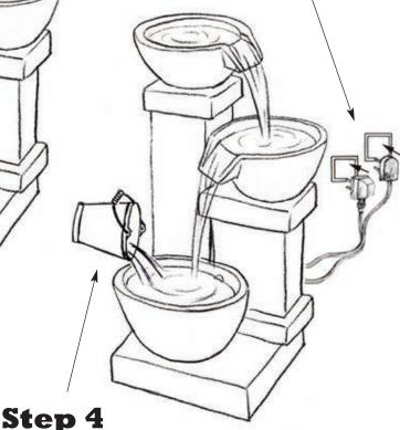
Fill the reservoir with water and take a note of the level that the water reaches for future reference when topping off.
