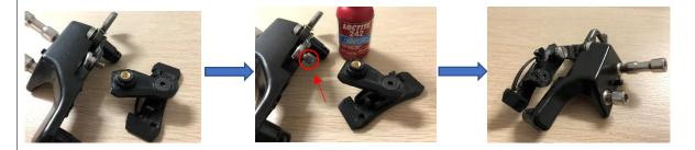
The Front Frame Spring is placed on the two metal sockets. Clean the sockets from any old plastic bits. The springs should have a tight fit without anything else needed.
