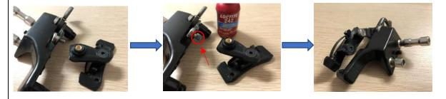
The *Front Frame Spring* is placed on the two metal sockets. Clean the sockets from any old plastic bits. The springs should have a tight fit without anything else needed.
