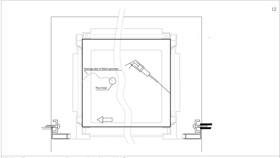
12. Use silicone to make a seal between the cabin and the floor. Get the steam drainlage pipe into the floor drain.
