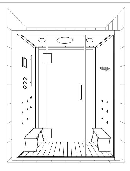
13. Put in the shower grid and seat. No using within 24 hours until the silicone is fully solid.
