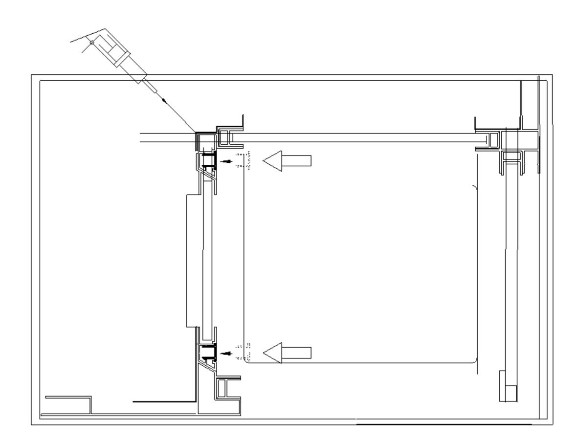
13. Get the aluminum profile in Apply silicone. No using within 24 hours
