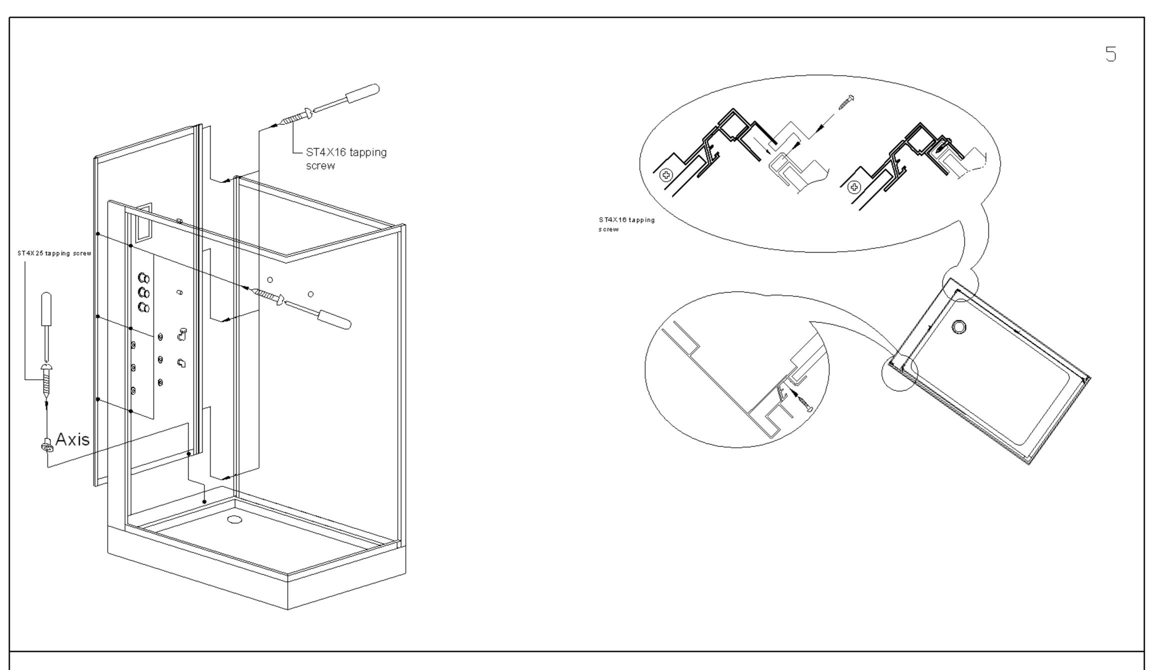
5. Install the back panel Get the back panel connected to the glass back wall with tapping screws.
