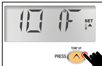
Press the “TEMP UP” or “TEMP DOWN” button to set desired temperature while the numbers are flashing
