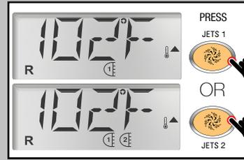
Press "JETS 1" button for pump 1 low speed to turn on. Press "JETS 2" button to activate pump 2 (if available)
