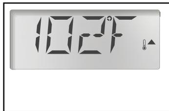
When the flashing stops, the temperature is set and will show the current temperature of the water
