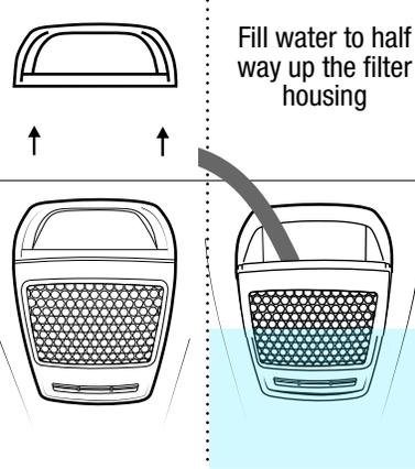
Remove the lid and fill the hot tub with water through the filter housing
