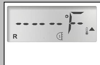
Pump 1 will then run on low speed to read current temperature. It will then start to heat up to the set temperature.
