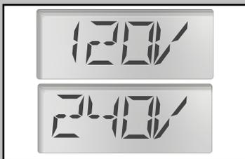
Make sure the voltage shown on your screen matches the electrical voltage of the hot tub (120V **OR** 240V)
