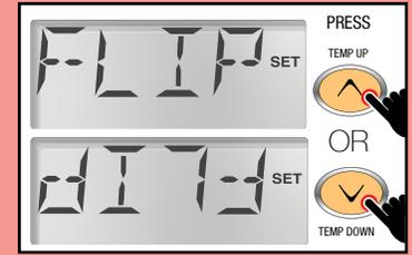
Press "TEMP UP" or "TEMP DOWN" button to set which orientation you would like for the screen to display. Press "MENU" again to complete action
