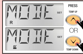
Press the "TEMP UP" or "TEMP DOWN" button to select Ready R or Rest Mode
