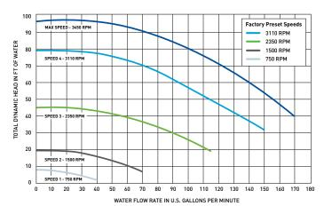
NOTE: The chart above demonstrates performance rates at factory preset speeds of 750 RPM, 1500 RPM, 2350 RPM and 3110 RPM.
