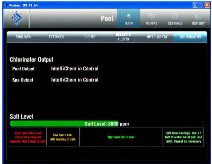
Chlorinator (IntelliChlor) with IntelliChem controller screen
