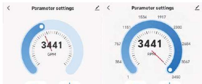
**In the Manual Mode,** just touch Speed 1, or 2, or 3, then you will enter the below setting pager. By moving the control bar, you can set flow & speed. You can set Maximum flow, but in the real situation, you can't reach the maximum flow because there are filters, elbows & other which will reduce the flow. The current flow rate will be shown at status bar.
