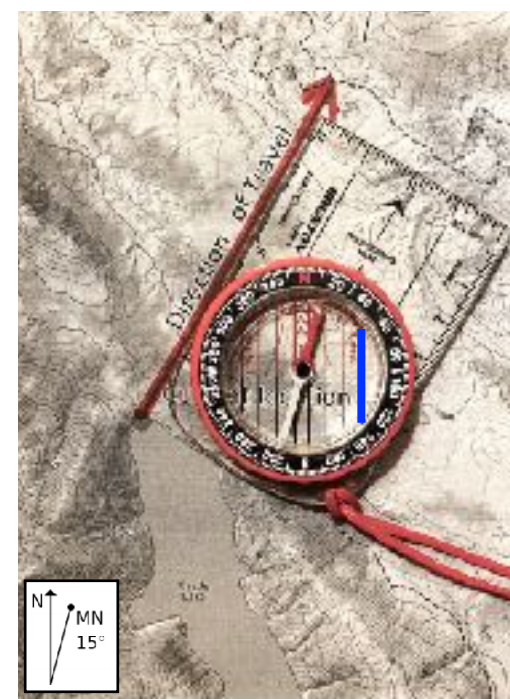
Finding a bearing: The north-south line (or edge of map) should parallel the orienting lines on compass. The blue lines serve to highlight how these parallel. In this example, the bearing for the direction of travel is 28°.
