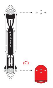
Place the Steadyrack on top of the Lock Bracket, aligning with the previous mounting holes (C). Replace the lower mounting screws (using the original screws) ensuring they go through both the Steadyrack and Lock Bracket (D).
