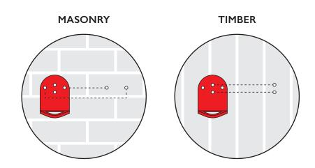
Place the new Lock Bracket over the lower mounting holes from your Steadyrack installation. The Lock Bracket has been designed to use the same mounting holes as the Steadyrack.
