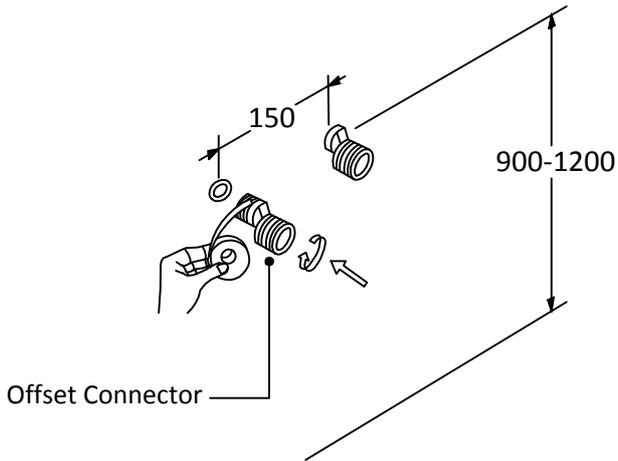
Apply PTFE tape to threads of offset connectors; connect offset connectors onto inlet pipes.
