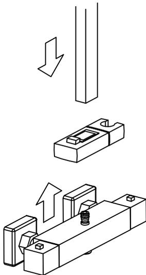
Install the riser into the top outlet of the shower valve.
