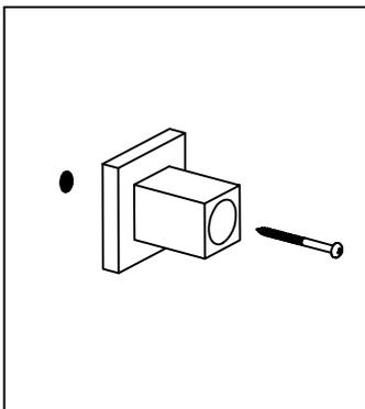
Drill the screw holes and install the wall plugs.
