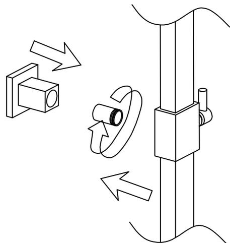
Fit the wall bracket to the riser kit
