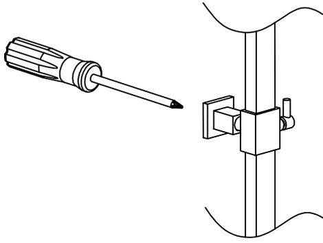
Make sure the riser is level, mark the position of the screw holes on the wall bracket.
