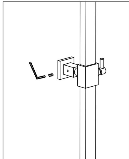
Install the riser on the wall bracket, tighten the screw.
