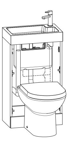
4. FIT PAN USING PAN FIXING KIT ONLY.
