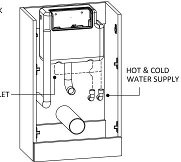
6. REFIT PANELS, CONNECTING FLUSH AND THEN SEAL WHERE REQUIRED.
