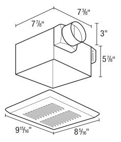
Acceptable for use over tub or shower when installed in a GFCI protected branch circuit.
