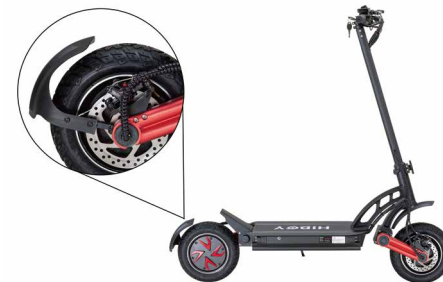
5. Remove the rear screws, install the rear fender then tighten the screws
