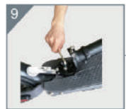
9. Tighten screw with a hexagonal wrench.
