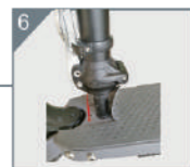
6. Insert the assembled seat into the hole on the scooter.
