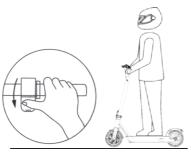
3. When the scooter starts to coast, put both feet on the deck and press the throttle (the throttle initiates once the coasting speed exceeds 3.1 mph).
