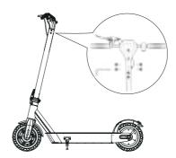
3. Use the Allen wrench to fix 6 screws, make sure it's tightened.
