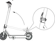
1. Unfold the stem and push the folding lever until you hear a click. Then unfold the kickstand to support the scooter.
