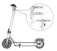
2. Attach the handlebar to the stem. Make sure it's right way round.
