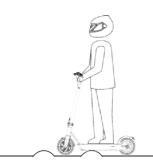
Keep your speed between 3.1-6.2 mph when you ride through speed bumps, elevator door sills, bumpy roads or other uneven surfaces. Slightly bend your knee to better adjust mentioned surfaces.
