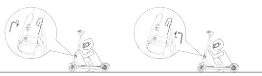
If the handlebar and its stem sway during riding, please tighten the screws on the folding mechanism.
