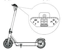
1. Turn the power on, and check the power indicator.
