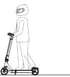
4. Release the throttle to reduce the speed slowly. Squeeze the brake lever for a sudden brake.
