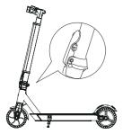
1. Unfold the stem and push the folding lever until you hear a click. Then unfold the kickstand to support the scooter.
