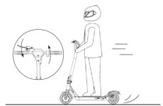
4. Release the throttle to reduce the speed slowly. Squeeze the brake lever for a sudden brake.
