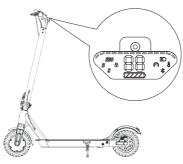
1. Turn the power on, and check the power indicator. Note: The scooter can not be turned on during charging
