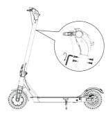
3. Use the Allen wrench to fix 6 screws, make sure it's tightened.
