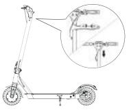
2. Attach the handlebar to the stem. Make sure it's right way round.
