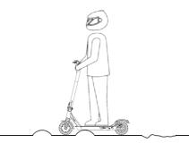
Keep your speed between 3.1-6.2 mph when you ride through speed bumps, elevator door sills, bumpy roads or other uneven surfaces. Slightly bend your knee to better adjust mentioned surfaces
