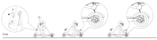
Make sure that the scooter's turned off. To fold, unlock the folding mechanism, and bend the handlebar stem to hook the clamp on the rear fender. To open, unhook from the clamp, erect the handlebar and lock the folding structure.
