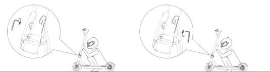
If the handlebar and its stem sway during riding, please tighten the screws on the folding mechanism.
