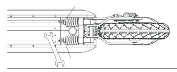
We have pre-adjusted the rear suspension to make it be workable for 165 lbs+ users, if you feel the suspension is too loosen or tight, then please use No. 14 wrench to adjust the two nuts on the suspension and make it more tight or loosen until you feel the suspension is working well for your weight.
