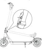
1. Unfold the stem and push the folding lever until you hear a click. Then unfold the kickstand to support the scooter.
