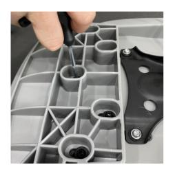
Insert 5 of the longer screws and install it with the Wrench.
