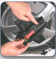
3. Tighten the snow chain with the belt tensioner.
