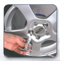
1. Bolt the fastening elements to 2 wheel nuts on each wheel rim.
