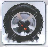
2. Mount the chain on the tyre and secure with the rail on the dual fastening system.
