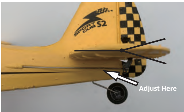
Elevator not properly centered.
