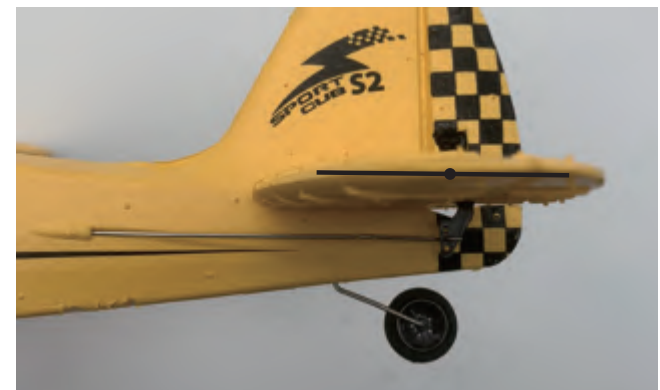
Elevator properly centered.
