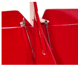
Typical elevator and rudder pushrod setups.
