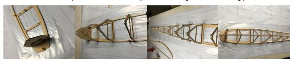
6. Enhance fuselage structure with 6x6mm balsa sticks
