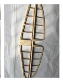
30. The horizontal tail is connected to the fuselage with a 3MM screw. It can be disassembled for easy transportation.
