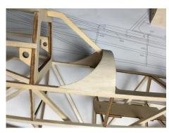
20.Paste A15 plywood onto the fuselage, and fill the nose with 5MM balsa sheet and polish it
