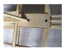
31. The wing ribs shall be assembled according to the position of the drawing. The balsa sticks of the main wing girder shall be 6X8MM, and need to be spliced and extended
