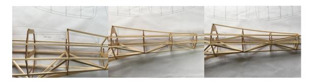
12. A35 plywood are pasted with round stiffeners and claw nuts and then combine the finished parts and the frame
