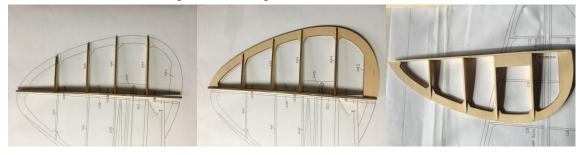
26. Paste 6X8MM balsa sticks and C12 plywood, assemble the wing ribs, paste the leading edge plywood, and paste 6X8MM balsa sticks on the leading edge of the tail fin and polish them
