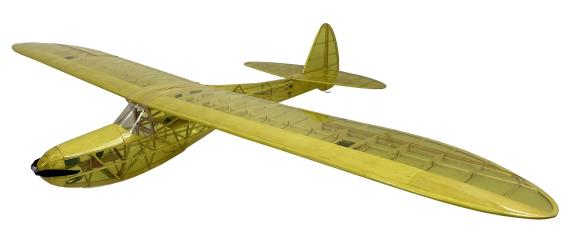
SB98 is a glider model airplane for relaxed flying. Low flying weight and wing load makes an awesome calm wind performer. The calm and silent flying characteristics attracts both intermediate and advanced pilots. SB98 can be built with or without electric power set.SB98 is controlled by rudder, elevator and ailerons.
