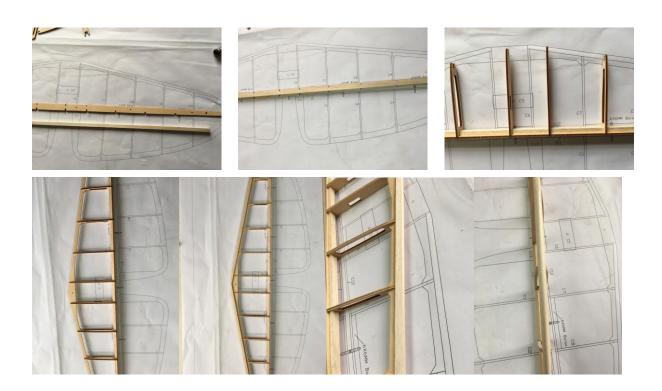
27. Paste two pieces of C5 to middle rib and use 2mm blasa sheet to paste the upper and lower covers
