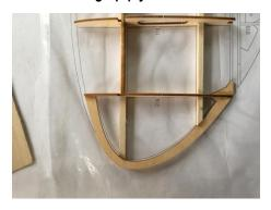
33. The back edge is pasted with 6X8MM balsa sticks and B20 plywood
