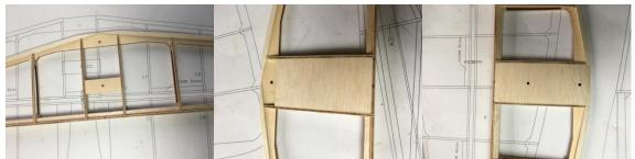
28. Compositely paste C11 and 8mm balsa stick, and the balsa sticks need to be spliced and extended
