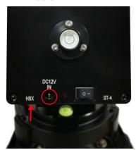
7. Set Zero Position: The Zero Position is the mount GOTO reference. Without setting the mount zero position properly, it may cause large GOTO error or even cause the scope to hit the tripod leg. The simplest way to find the mount Zero Position of the EQ mode is using the zero position sensors. Press MENU=>Zero Position =>Search Zero Position, then
