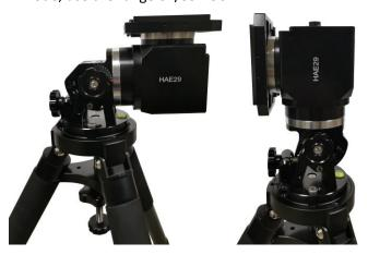
5. <u>Install telescope</u>: HAE29 accepts a Vixen or a Losmandy-D dovetail mounting bar. The default is Vixen-type one. Release the dovetail Saddle Locking Screws and slide the telescope dovetail plate into the saddle. Make sure that the arrow sign on the saddle is pointing forward. Tighten the Saddle Locking Screws.
