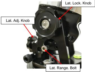
Use the Latitude Adjustment Knob to move the mount to a proper Latitude Range and thread in the Latitude Range Bolt. Fine adjust the latitude to corrected latitude. Here the mount is set at 40°. Tighten the Latitude Locking Knob.
