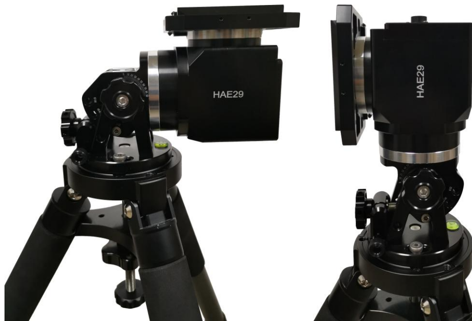
Figure 14. An HAE mount set for equator ( 0^{\circ} , left) and altazimuth ( 90^{\circ} , right) use
