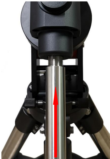
Figure 20. Install CW shaft
