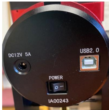
Figure 7. GEM45 Power Panel on Rear of RA axis
