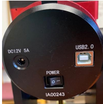
Figure 3. GEM45 Power Panel on Rear of RA axis
