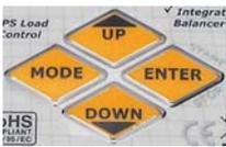
**MODE:** Before Charging/Discharging is started: Scrolls between MENUS for MEMORY (Charging), USER SETUP, DATA VIEW, BALANCER.
