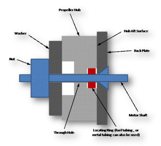
In addition to the supplied Locating Rings (electric propellers only), aluminum tubing and/or fuel tubing can be used to center the propeller on the shaft. The standard through hole diameters for APC propellers are 3/16", 1/4", and 5/16".
