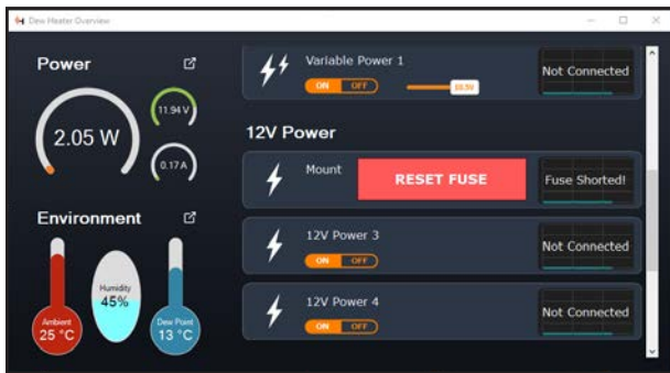
Fig 15 If the power draw on a port exceeds the maximum for the port, then the port will automatically shut off. To re-enable the port, click the RESET FUSE box once the load on the affected port has been reduced.
