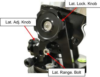
Use the Latitude Adjustment Knob to move the mount to a proper Latitude Range and thread in the Latitude Range Bolt. Fine adjust the latitude to corrected latitude. Here the mount is set at 40°. Tighten the Latitude Locking Knob.
