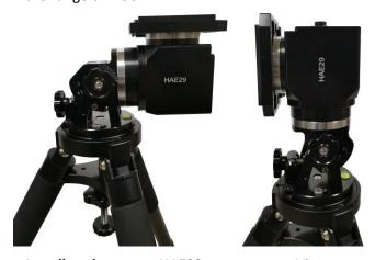
5. <u>Install telescope</u>: HAE29 accepts a Vixen or a Losmandy-D dovetail mounting bar. The default is Vixen-type one. Release the dovetail Saddle Locking Lever and slide the telescope dovetail plate into the saddle. Make sure that the arrow sign on the saddle is pointing forward. Tighten the Saddle Locking Screw.
