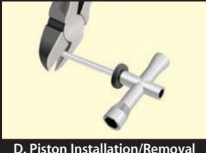
D. Piston Installation/Removal
