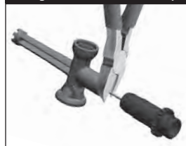
C. Remove/Install Rod End
