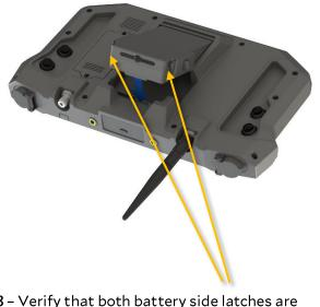
3 – Verify that both battery side latches are fully engaged with the TAC housing to securely capture the battery!
