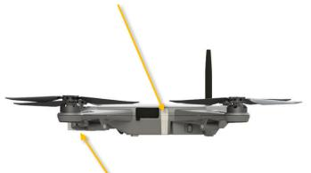
4 - Verify gimbal start-up, indicated by its movement to a properly-centered, level, and forward-facing position.
