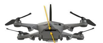
2 - Verify that the center LED is lit, indicating battery power is on.
