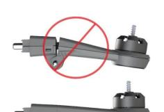
Check that props are not damaged. Replace if nicked, warped, or cracked!
