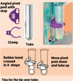
If the tip-over tube doesn't rotate in the correct direction check to make sure that you have the clamp attached to the pivot post correctly. If it doesn't tip over at all, try moving the angled pivot post down one peg on the tower, and positioning the tube higher up in the clamp. Also, experiment with starting with different numbers of gumballs in the tube.
