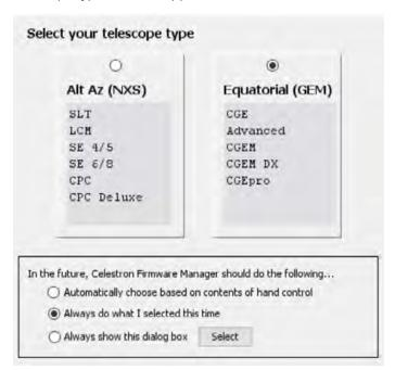
Find your mount and click on the corresponding "Alt Az (NXS)" box or "Equatorial (GEM)" box. Then, click on the "Always do what I selected this time" selection at the bottom of this window. Next, click the Select box at the bottom of the window to confirm your selections, and the window will close.
