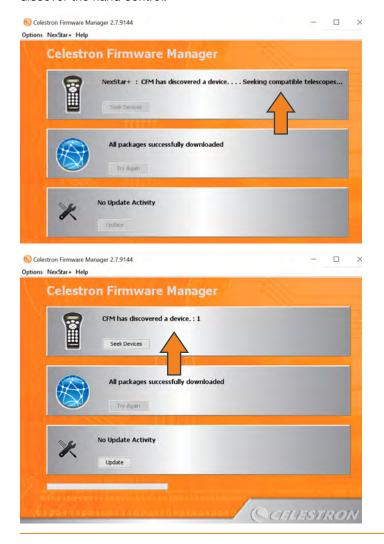
If CFM does not discover the hand control automatically, check your cable connections and press "Seek Devices" in CFM. When CFM finds the hand control, the hand control will display "BOOT LOADER Serial Pass Through OFF."
