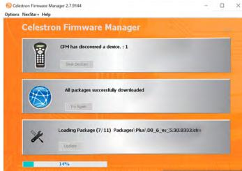
**WARNING:** Do not disconnect the hand control or power off the computer or mount while the update is in progress!
