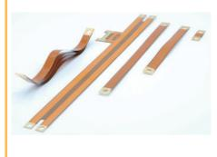
Flexible Printed Cable is made by applying printed circuit board manufacturing technology to laminate conductor and insulation materials. In general cables, the skin effect occurs during AC conduction, causing the resistance value to rise. This unique multilayered structure brings better skin effect and provides a higher power supply capacity. Also low inductance can be achieved due to the canceling effect of the magnetic field by the multilayer structure.
