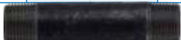
3/4" DIAMETER DIAMETER BLACK EXTRA HEAVY XXS SEAMLESS Wall Thickness 0.308 - Grade B - Test Pressure 1000 PSI - Thread Length 0.79
