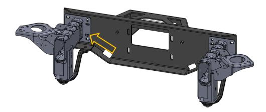
21. Install the passenger and driver side Frame Reinforcement Brackets onto the back of the frame horn over the 3/8" stud followed by a flat washer, lock washer and nut. Snug the nuts up tight enough that there is no slop in the connection, but so the bracket can still be moved around.
