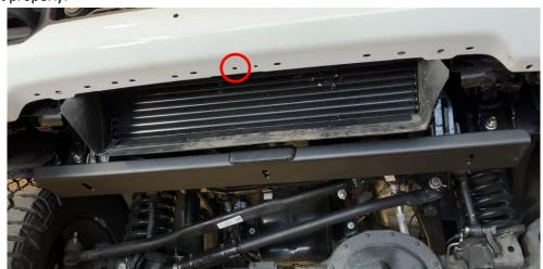
7. Install the M8 U-nut onto the front bumper with the threaded boss facing upwards.
