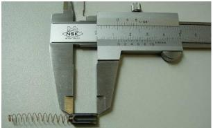
Measure length of carbon brush Check contact surface for scorch marks (if a "carbon brush jam" is detected replace carbon brushes as well as carbon brush supports)
