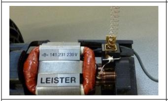
Re-insert carbon brushes in the same fitting positions. Press springs in brush supports and bend ears to closed positions
