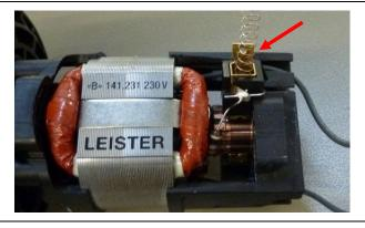
Carefully bend up the ear of the carbon brush support and remove carbon brush Caution, spring is under tension!
