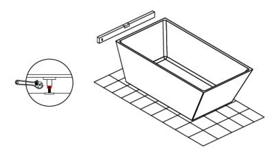
5. Align and connect the tub's drain to the waste drain outlet.
