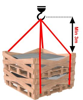
THE LIFTING HOOK SHOULD BE NO LESS THAN 3M ABOVE THE LID
