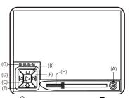
(A) Open File : Press the button of □ (Camera) in the mode of Video Play to enter the interface of file selection. Select the demanded file as in the following image. After selection, press the button of □ to play. Use buttons of □ and □ to select items in the interface (such as file type, file slot, file folder and file). Use buttons of □ and □ to select options in the interface.
