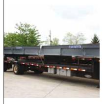
The premium portable design can be moved in one piece. Simply lift the scale and its attached frame onto a flat-bed trailer for transport. The basic portability option requires removing the scale modules and dismantling the frame before loading the components onto a trailer to be moved.
