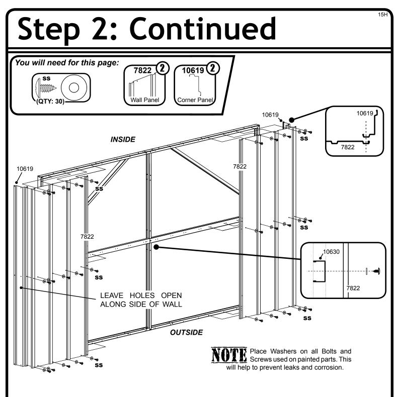
Using **Small Screws**, attach a **Wall Panel** and **Corner Panel** to each corner of the **Rear Wall** as shown. The **Corner Panel** should only be secured to the **Wall Panel** where the **Panels** overlap. Do not secure the **Corner Panel** to the **Rear Wall** itself, this will be done in Step 5.
