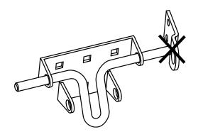
If Slide Bolt does not align properly, you may need to insert plastic washers between the door and the Slide Bolt to ensure proper fit. Adjust number of plastic washers until desired fit is reached.
