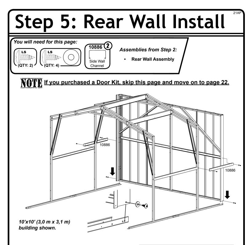
Carefully position the **Rear Wall Assembly** in place at the rear of the building and secure to **Side Frame** with one **Large Screw** per side as shown.
