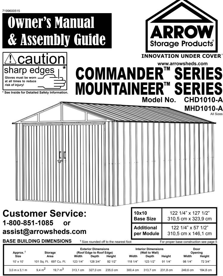
Each Module adds an additional 57 1/2" (146,1 cm) in length, 47.2 Sq. Ft. (4,4 m<sup>2</sup>) additional storage area, and 324 Cu. Ft. (9,2 m<sup>3</sup>) additional storage volume.
