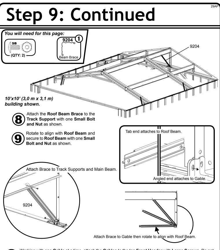
Working with one **Gable** at a time, attach the **Gables** to the top **Front Header** with **Large Screws**. Do not insert screws into the two holes closest to where the **Gables** join. These will be used to attach the **Track Support** later. Repeat Steps 9-3 thru 9-9 to install **Gables** at the front of the building.
