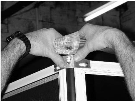
**C.** Tighten the nut on the tube tips to maintain a small amount of tension.
